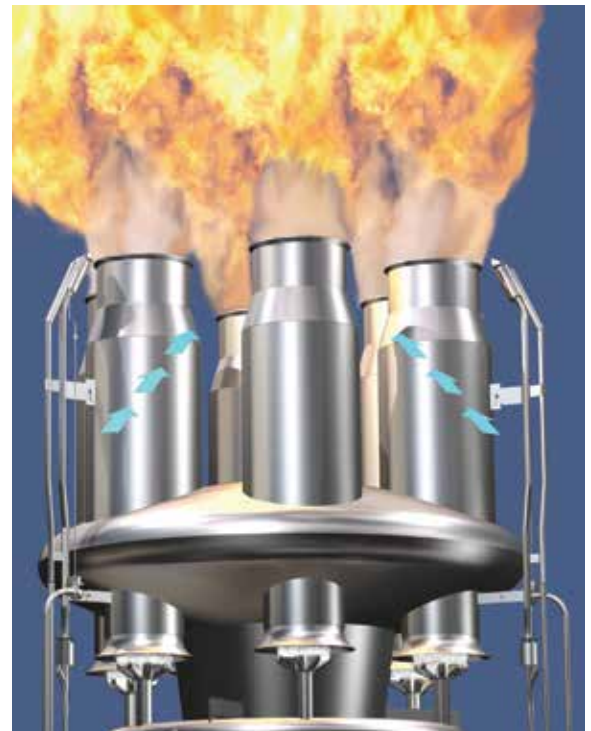
SECONDARY AIR ENTRAINMENT
